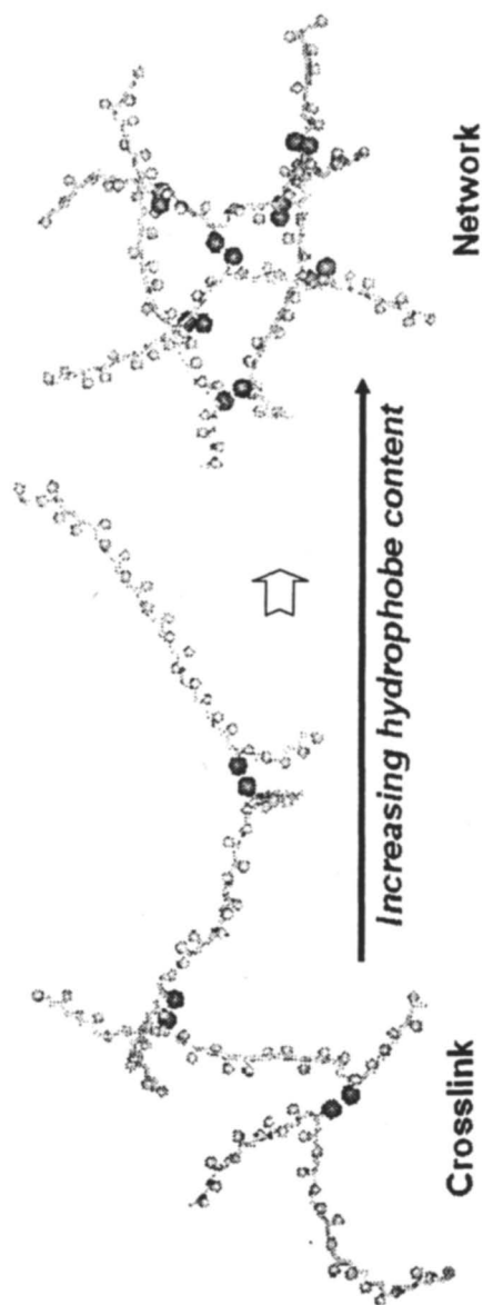
Figure 3. Completely Interpolymer associations of hydrophobes forming crosslinks.
